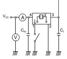
$C_L$ ; 15pF MAX including input capacity of oscilloscope  $C_{bv}$ ; Bypass capacitor (0.01uF)
